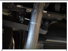
3. Install the overaxle pipe into the muffler outlet no less then 1.5". Please note when using the clamp it needs to be place to the furthest point of the muffler outlet to grab both pipes.
