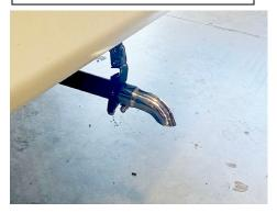
7. To Install the Generator turn down tip. Simply hold the tip up to your factory exhaust and mark the end of the tip. Add 1.5" to the mark towards the end of the exhaust and cut. Be sure the tip still extends past your body panel 1.5".
