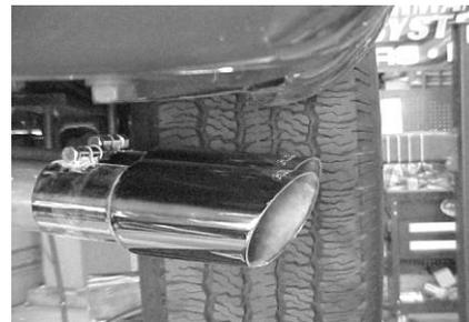
INSTALL TAILPIPES#C, D USING CLAMP#G TO ATTACH TO MUFFLER. BOLT KIT#H TO CONNECT BOTH THE TAILPIPES TOGETHER. THE TAB ON THE DRIVERSIDE TAILPIPE WILL BE ON TOP. TIGHTEN ALL CLAMPS AND HANGERS. NOW INSTALL YOUR STAINLESS STEEL TIPS TO YOUR DESIRED LOOK. USE ANY ALUMINUM OR STAINLESS STEEL CLEANER TO POLISH YOUR TIP.
