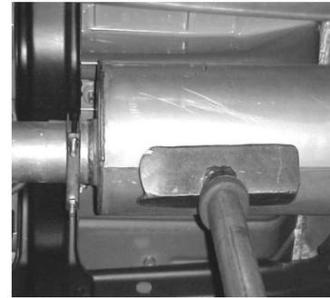
LAYOUT THE GIBSON EXHAUST AS SHOWN ON YOUR MANUAL. COMPARE THE PIPE NUMBERS TO THE MANUAL NUMBERS. MAKE SURE THEY ALL MATCH. THEN, CUT THE STOCK TAILPIPE OFF JUST AFTER THE MUFFLER FOR EASY REMOVAL. AFTER CUTTING THE TAILPIPE, UNBOLT THE STOCK HEADPIPE AND REMOVE THE WHOLE SYSTEM. LEAVE ALL RUBBER GROMMETS IN PLACE. **YOU WILL REUSE STOCK FLANGE BOLTS AND GASKETS.**
