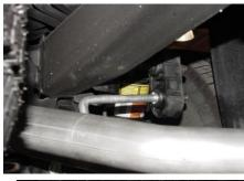
INSTALL PASSENGER SIDE OVERAXLE TAILPIPE # D INTO MUFFLER 1-1/2" TO 2" . INSERT WELDED HANGER INTO RUBBER GROMMET. USE CLAMP # H TO SECURE PIPE TO MUFFLER. DO NOT TIGHTEN.
