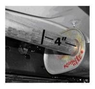
TO REMOVE STOCK EXHAUST MEASURE 4" FROM THE FRONT OF THE MUFFLER FORWARD AND CUT. NOW CUT OFF YOUR STOCK TAILPIPE JUST BEHIND THE MUFFLER AND REMOVE. LEAVE ALL RUBBER GROMMETS ON THE HANGER. USE WD-40 TO AID IN THE REMOVAL OF THE EXHAUST AND HANGERS.
