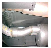
INSTALL HEADPIPE # A SLIP IT ONTO STOCK HEADPIPE USING CLAMP # K TO SECURE IT. INSERT WELDED HANGER INTO RUBBER GROMMET. DO NOT TIGHTEN. INSTALL HEADPIPE # B, SLIP IT ONTO THE STOCK HEADPIPE USING CLAMP # K TO SECURE THE HEADPIPE TO THE STOCK PIPE. DO NOT TIGHTEN.
