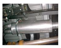
3. INSTALL BAND CLAMP # G INTO RUBBER GROMMETS LOCATED ABOVE THE REAR AXLE. DO NOT TIGHTEN. INSTALL MUFFLER # B THROUGHT BAND CLAMP AND ONTO HEADPIPE. USE CLAMP # L TO SECURE MUFFLER TO HEADPIPE. DO NOT TIGHTEN.
