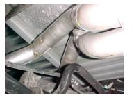
4. INSTALL DRIVERS SIDE OVER AXLE TAILPIPE # C INTO MUFLER 1 1/2" TO 2" USE CLAMP # H TO SECURE PIPE TO MUFFLER. DO NOT TIGHTEN.
