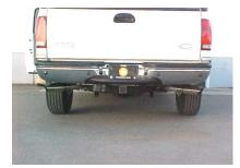
6. MEASURE 18 ½" FROM THE REAR OF THE FRAME YOU WILL USE THIS SLOT FOR YOUR 10" HANGER. USE THE 3<sup>RD</sup> HOLE FROM THE TOP. USE CLAMP # H TO HOLD TAILPIPE # C TO HANGER. DO NOT TIGHTEN.
