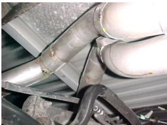
4. INSTALL DRIVERS SIDE OVER AXLE TAILPIPE # C INTO MUFLER 1 1/2" TO 2" USE CLAMP # H TO SECURE PIPE TO MUFLER. DO NOT TIGHTEN.
