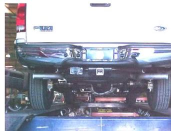
7. INSTALL TURNOUT PIPES # E ONTO BOTH TAILPIPES. ROTATE TILL LEVEL . USE CLAMP #H TO SECURE EXITPIPES TO TAILPIPES AFTER CHECKING FOR PROPER CLEARANCE. TIGHTEN ALL CLAMPS STARTING FROM THE FRONT AND WORKING YOUR WAY BACK.
