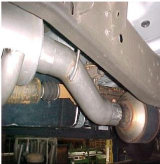
2. INSTALL HEADPIPE #A ONTO STOCK HEADPIPE, LINE UP THE NOTCH AND INSERT WELDED HANGERS INTO RUBBER GROMMETS USE CLAMP # K TO SECURE PIPES TOGETHER. DO NOT TIGHTEN. LEAVE LOOSE FOR EASIER INSTALLATION.
