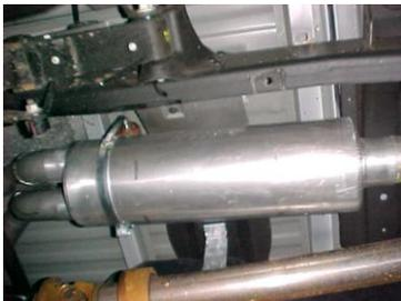
3. INSTALL BAND CLAMP # G INTO RUBBER GROMMETS LOCATED ABOVE THE REAR AXLE AND ATTACH WITH BOLT KIT #M. DO NOT TIGHTEN. INSTALL MUFLER # B THROUGH BAND CLAMP AND ONTO HEADPIPE. USE CLAMP # L TO SECURE MUFLER TO HEADPIPE. DO NOT TIGHTEN.
