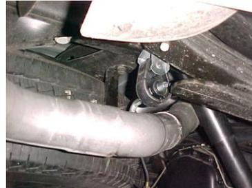
5. INSTALL PASSENGER SIDE OVERAXLE TAILPIPE # D INTO MUFLER 1 1/2" TO 2" INSERT WELDED HANGER INTO RUBBER GROMMET. USE CLAMP # H TO SECURE PIPE TO MUFLER. DO NOT TIGHTEN.
