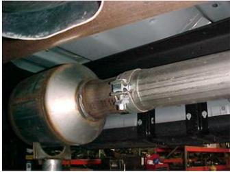
1. **TO REMOVE STOCK EXHAUST UN-BOLT IT FROM THE CLAMP LOCATED JUST BEHIND THE CATALYTIC CONVERTER.** CUT OFF YOUR STOCK TAILPIPE AND REMOVE. LEAVE ALL RUBBER GROMMETS IN PLACE. USE WD-40 TO AID IN REMOVAL OF EXHAUST AND HANGERS.
