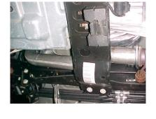
INSTALL PIPE #K N ONTO PIPE # OJ. USE CLAMPS #K TO SECURE PIPES TOGETHER. DO NOT TIGHTEN.
