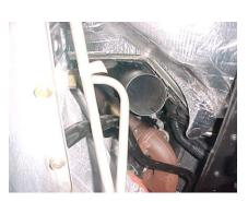
INSTALL PIPE # 0 ONTO TURBO RE- USING YOUR STOCK CLAMP. DO NOT TIGHTEN.
