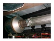
1. TO REMOVE STOCK EXHAUST UN-BOLT IT FROM THE CLAMP LOCATED JUST BEHIND THE CATALITIC CONVERTER. CUT OFF YOUR STOCK TAILPIPE AND REMOVE. LEAVE ALL RUBBER GROMMETS IN PLACE. USE WD-40 TO AID IN REMOVAL OF EXHAUST AND HANGERS.
