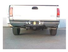
8. INSTALL THE STAINLESS TIPS FOR YOUR DESIRED LOOK. TO CLEAN TIPS, USE A SCOTCH BRITE PAD AND ANY STAINLESS STEEL OR ALUMINUM CLEANER.
