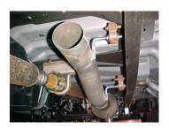
2. INSTALL HEADPIPE #A ONTO STOCK HEADPIPE, LINE UP THE NOTCH AND INSERT WELDED HANGERS INTO RUBBER GROMMETS USE CLAMP # K TO SECURE PIPES TOGETHER. DO NOT TIGHTEN. LEAVE LOOSE FOR EASIER INSTALLATION.
