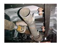
1. INSTALL HEADPIPE #A ONTO STOCK PIPE, LINE UP THE NOTCH AND INSERT WELDED HANGERS INTO RUBBER GROMMETS USE CLAMP # K TO SECURE PIPES TOGETHER. DO NOT TIGHTEN.
