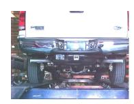
6. INSTALL TURNOUT PIPES # E ONTO BOTH TAILPIPES., ROTATE UNTIL LEVEL . USE CLAMP #H TO SECURE PIPES TO TAILPIPE AFTER CHECKING FOR PROPER CLEARENCE. TIGHTEN ALL CLAMPS STARTING FROM THE TURBO AND WORKING YOUR WAY BACK.
