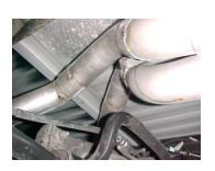
3. INSTALL DRIVERS SIDE OVER AXLE TAILPIPE # C INTO MUFLER 1 ½" TO 2" USE CLAMP # H TO SECURE PIPE TO MUFFLER. DO NOT TIGHTEN.
