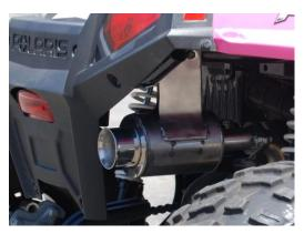
3. Install muffler #B using factory bolts then attach both pieces together with provided hardware. Tighten all nuts and bolts.
