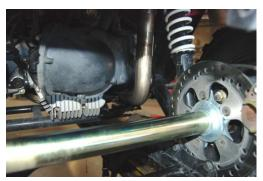
2. Install Headpipe #A using factory nuts. Leave nuts loose.
