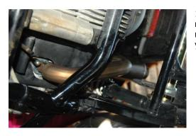
1. Remove your stock exhaust by removing the two bolts holding the muffler on. Do Not discard these bolts. You will re-use them. Next remove the two nuts from the cylinder head. Do Not discard these nuts as you will re-use them also.
