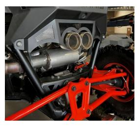
4. Next install the Gibson Beauty Plate #B using the 2 Factory Torx Bolts. With everything installed and now tight be sure to double check clearance of O2 wire and all other parts. We need a minimum of 1" of clearance. It is important that all parts are cleaned of grease, finger prints, and any sport of liquid to prevent staining. Re connect the battery cable and enjoy your new Gibson exhaust.
