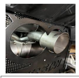
5. Now, install passenger side tip #F by fishing it through the beauty plate very carefully. Use clamp # G to secure to pipe. (DO NOT TIGHTEN)
