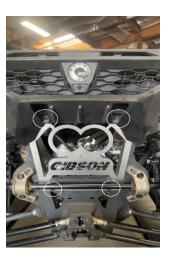
3. Next, install the beauty plate on the vehicle using the 4 existing bolts on the rear fascia.
