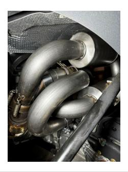
6. Once the passenger tip is installed you may install the intermediate pipe #D into the E-Valve #C using clamp #G (DO NOT TIGHTEN)
