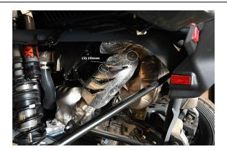
2. To remove the factory muffler, you'll need to remove the heatshield covering the head pipe which is held on by( 3) 10mm bolts. Then, remove the ( 4) springs holding on the exhaust head pipe and the 4 bolts holding the muffler to the frame of the vehicle located beneath the muffler assembly.
