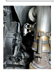
4. Then, install E-Valve #C onto headpipe with clamp #G (Be sure the electronic portion is parallel to electric fan shroud. DO NOT TIGHTEN.
