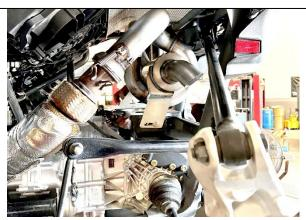
3. Finally, install muffler assy #A by fishing it through the passenger side wheel well. (BE CAUTIOUS AND PATIENT WHEN FISHING IT THROUGH AS IT IS A TIGHT FIT.) Once in place reinstall the 4 bolts that secure the muffler loosely then install all 4 springs to the head pipe, once springs are installed go back and tighten the 4 bolts securing the muffler.
