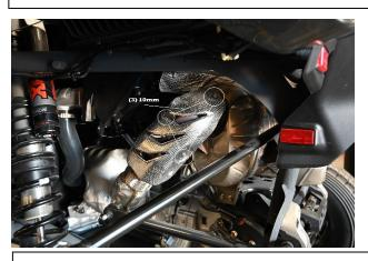
2. To remove the factory muffler, you'll need to remove the heatshield covering the head pipe which is held on by 3 10mm bolts. Then, remove the 4 springs holding on the exhaust head pipe and the 4 bolts holding the muffler to the frame of the vehicle located beneath the muffler assembly.
