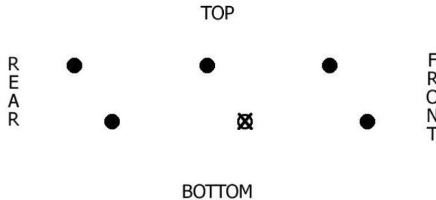
6. Now install passenger side GIBSON header, gasket, stock hardware, the supplied 8mm bolt and washer to the head and torque the header to 30-35 ft/lb.
