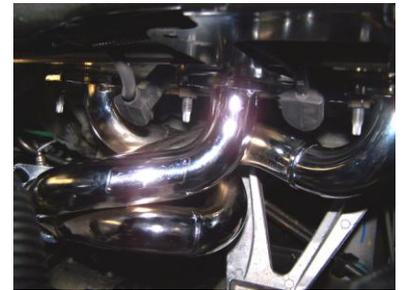
7. Re-install Y-pipe assembly to the GIBSON headers and torque to 30-35 ft/lb.
