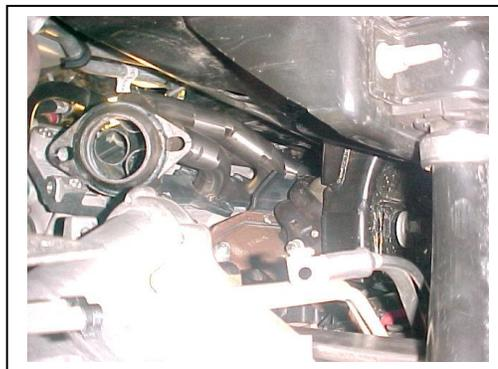
14. RE-CONNECT THE EXHAUST SYSTEM TO THE NEW HEADERS USING THE HARDWARE PROVIDED.(RE-CONNECT DRIVE SHAFT WHERE APPLICABLE)
