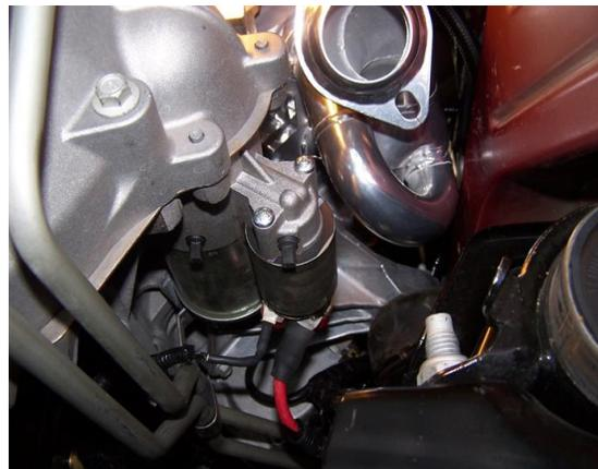
17. RE-CONNECT THE EXHAUST SYSTEM TO THE NEW HEADERS USING THE HARDWARE PROVIDED.
