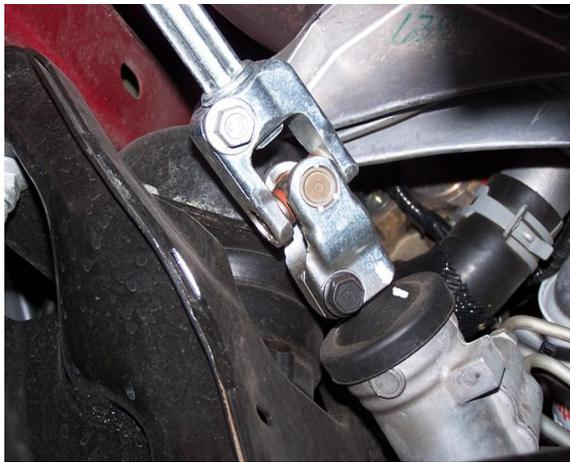
3. SPRAY WD-40 OR SOME TYPE OF PENETRATING OIL ON ALL ACCESSIBLE FASTENERS AND FITTINGS BEFORE ATTEMPTING TO REMOVE THEM.
