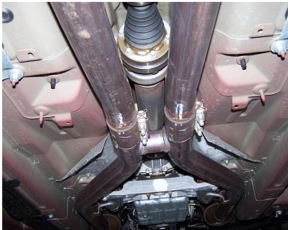
5. DISCONNECT ALL O2 SENSORS. THEN FROM UNDERNEATH THE VEHICLE, LOOSEN THE BOLTS CONNECTING THE Y-PIPE ASSEMBLY TO THE EXHAUST MANIFOLD.
