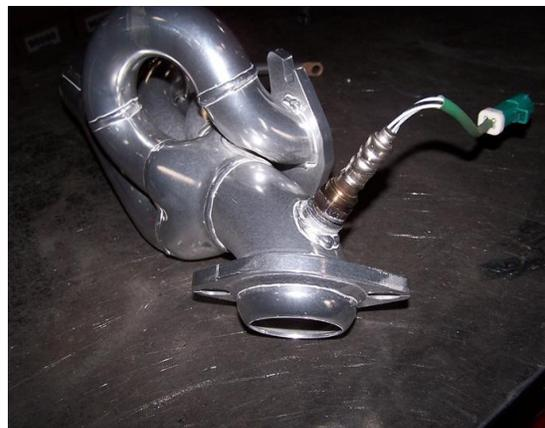
12. BEFORE INSTALLING DRIVER SIDE HEADER, REMOVE O2 SENSOR FROM FACTORY MANIFOLD AND RE-INSTALL IN YOUR NEW HEADER. USE ANTI-SIEZE ON THE THREADS OF THE O2 SENSOR.
