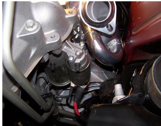
TORQUE DOWN BOLTS STARTING WITH THE CENTER BOLTS FIRST. RECOMMENDED TORQUE SPECS. ARE 25-30 FOOT POUNDS OF TORQUE.
