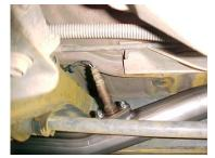
7. AFTER HOOK-UP OF HEADER & Y-PIPE ASSEMBLY LET IT COOL DOWN AND RETORQUE HEADER AND Y-PIPE ASSEMBLY TO PREVENT LEAKS.
