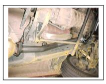
6. AFTER HEADPIPE IS INSTALLED USE 2 <sup>1</sup>/<sub>2</sub>" CLAMP AND CLAMP HEADPIPE TO STOCK MOUNTING BRACKET. THEN INSTALL FACTORY 02 SENSOR IN HEADPIPE. DOUBLE CHECK FOR CLEARANCE ON HEADPIPE AND TORQUE TO 35 FTS.
