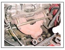
3. NOW BACK UP TOP REMOVE EGR RACK THEN REMOVE MANIFOLD AND STOCK GASKETS. CLEAN HEAD SURFACE USING GASKET SCRAPER. THEN INSTALL SUPPLIED GASKET AND GIBSON HEADER, MAKE SURE TO INSTALL 2 BOLT GASKET IN MIDDLE OF CYLINDER HEAD. TORQUE HEADER TO 35 FTS.
