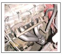
4. NOW STARTING UNDERNEATH PUT IN SUPPLIED DONUT GASKET IN BOTTOM OF HEADER.
