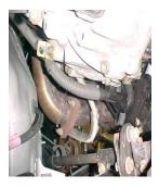
STARTING FROM UNDERNEATH THE VEHICLE LOOSEN FASTENERS ATTACHING THE Y-PIPE TO THE EXHAUST MANIFOLD DISCONNECT. Y-PIPE ASSEMBLY FROM IN FRONT OF CATALYTIC CONVERTER AND BOTH EXHAUST MANIFOLDS.
