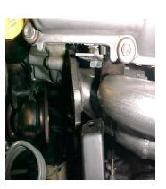
INSTALL SUPPLIED TRANSMISSION BRACKET EXTENSION FOR DIPSTICK MOUNT THAT BOLTS TO LAST UPPER LEFT HAND.BOLT ON PASSENGER SIDE (EXTENDS AWAY FROM HEADER TUBE)! ALSO USE SUPPLIED HEAT WRAP ON A/C LINE TO PROTECT FROM HEAT DAMAGE.
