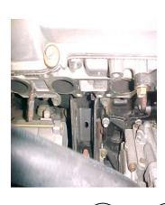
REMOVE THE STOCK STUDS WITH X'S THREW THEM FOR INSTALL.THEY ARE SUPPLIED 10MM BOLTS FOR INSTALL. SEE ILLUSTRATION BELOW.
