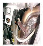
JUST LET Y-PIPE ASSEMBLY HANG OUT OF THE WAY. MAKE SURE TO SAVE FACTORY GASKETS; THEY WILL BE USED LATER IN THE INSTALLATION OF THE HEADERS.
