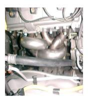
NOW START ON PASSAGNER SIDE REMOVE ANY BRACKETS FOR REMOVAL OF MANIFOLD. NOW REMOVE STOCK HARDWARE AND MANIFOLD MAKING SURE TO CLEAN HEAD SURFACE FOR INSTALLTION OF GIBSON HEADER.
