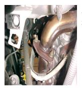
JUST LET Y-PIPE ASSEMBLY HANG OUT OF THE WAY. MAKE SURE TO SAVE FACTORY GASKETS; THEY WILL BE USED LATER IN THE INSTALLATION OF THE HEADERS.
