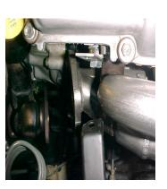
INSTALL SUPPLIED TRANSMISSION BRACKET EXTENSION FOR DIPSTICK MOUNT THAT BOLTS TO LAST UPPER LEFT HAND.BOLT ON PASSENGER SIDE (EXTENDS AWAY FROM HEADER TUBE)! ALSO USE SUPPLIED HEAT WRAP ON A/C LINE TO PROTECT FROM HEAT DAMAGE.
