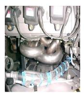
NOW INSTALL SUPPLIED HEADER GASKET, AND HEADER USING STOCK HARDWARE ON HEADER, TORQUING HEADER TO 30 TO 35 FTS. REINSTALL ANY BRACKETS TO CYLINDER.
